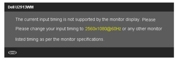
This means that the monitor cannot synchronize with the signal that it is receiving from the computer. See <u>Monitor Specifications</u> for the Horizontal and Vertical frequency ranges addressable by this monitor. Recommended mode is 2560 x 1080.
